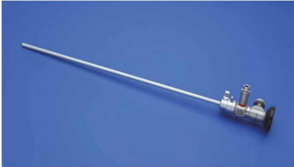
Fig. 1. This rigid scope was used as a salpingoscope (Karl-Storz, Germany). The diameter was 2.9mm, and maximum magnification was \times 60 .
