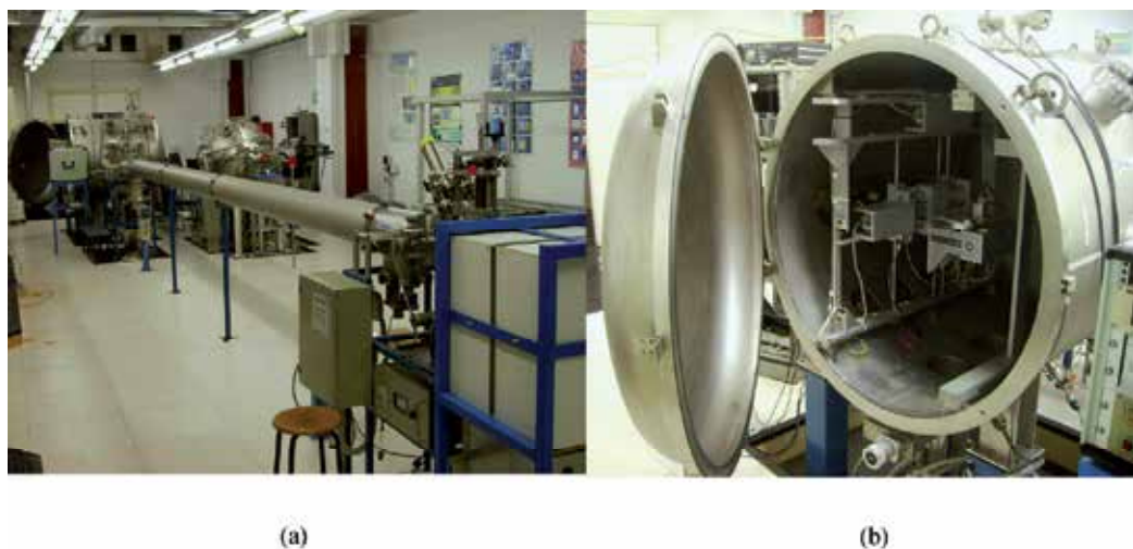
Fig. 7. (a) An overview of the LAX facility. (b) The detector chamber located at 10.5 m from the X-ray tube; the detection system was mounted on a XYZ microtranslator system.
