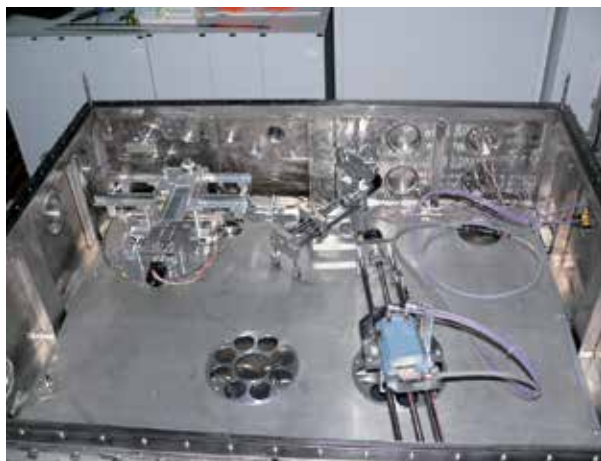
Fig. 2. Inside view of the J. Stefan Institute's WDX spectrometer vacuum chamber with the target holder on a goniometer, crystal holder, and the CCD camera. A mechanical \theta/2\theta stage serves to adjust the Bragg angle.
