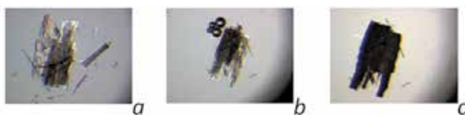
Fig. 13. HSM images for 4 at a) 25 °C; b) 140°C – water being released in the lactamization process; c) 144.5°C – crystal appearance just before melting 84 .
