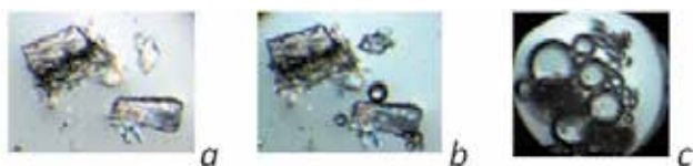
Fig. 14. HSM images for 5 at a) 25 °C; b) 90°C – slow release of crystallization water; c) 160°C – lactamization and melting 84 .
