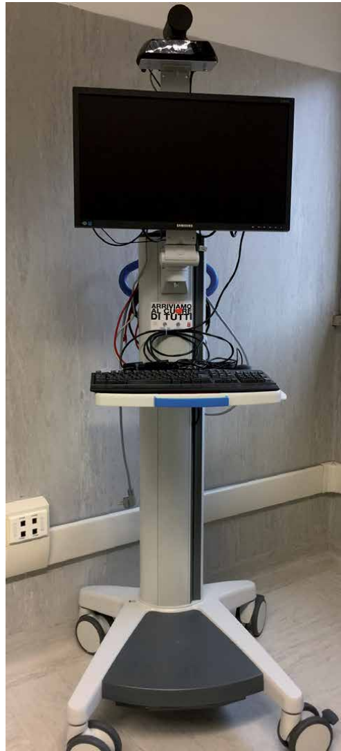
Figure 3. Mobile medical-grade cart, equipped with videoconferencing and computer workstation, allowing use in clinical setting.
