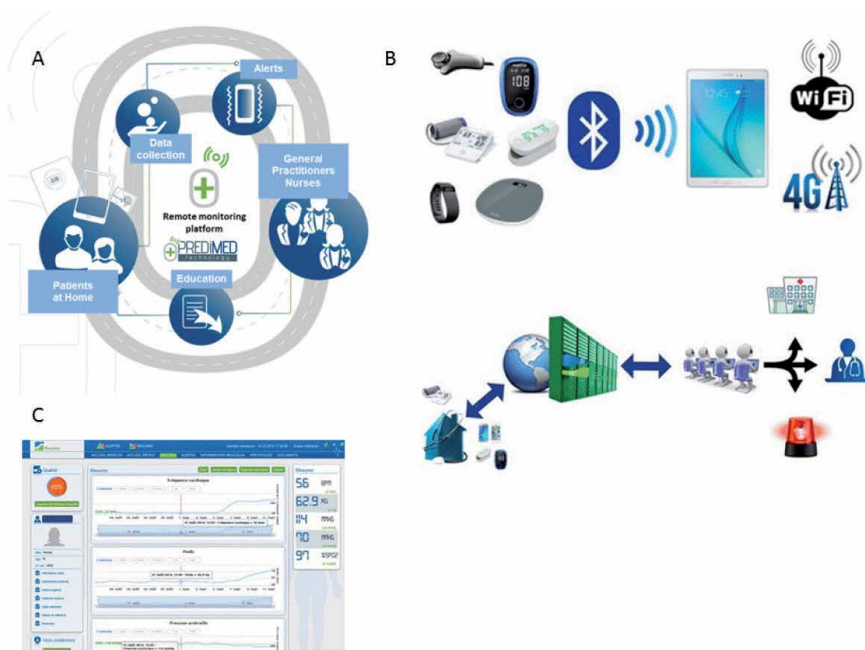
Figure 8. Intelligent telemonitoring project on diabetes and/or chronic heart failure management. (A) The system is based on an inference engine and a medical ontology for personalized synchronous or asynchronous analysis of data specific to each patient and, if necessary, the sending of an artificial intelligence-generated alert (MyPredi™). (B) The platform comprises connected noninvasive medical sensors, a touchscreen tablet connected by Wi-Fi, and a router or 3G/4G, rendering it possible to interact with the patient and provide education on treatment, diet, and lifestyle. (C) The system involves a server that hosts the patient's data and a secure Internet portal to which the patient and hospital- and non-hospital-based healthcare professionals can connect.
