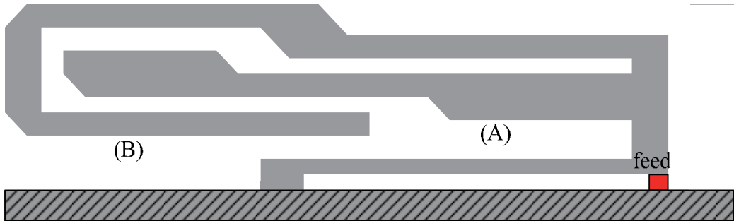
Fig. 5. A dual band inverted-F main resonator.
