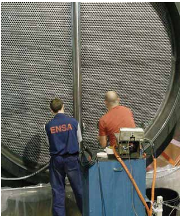
Fig. 1. Tubesheet of a steam generator for the nuclear industry
