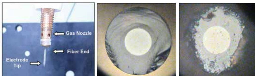
Fig. 9. Optical fibre embedded in a TIG welding torch (left), and view of the fibre's end before and after more than 100 welding trials
