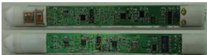
Fig. 11. Photograph of the new probe, front side (above) and rear side (bottom)
