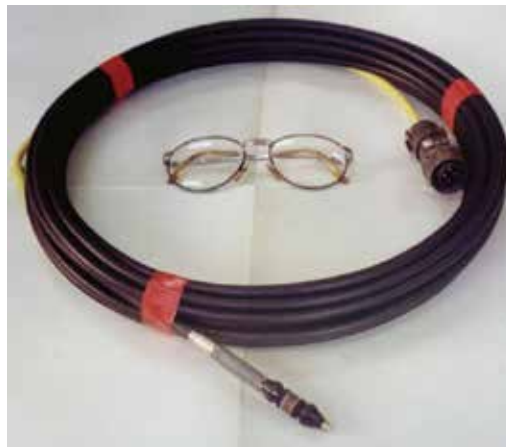
Fig. 14. EC probes for heat exchanger tube inspection.
