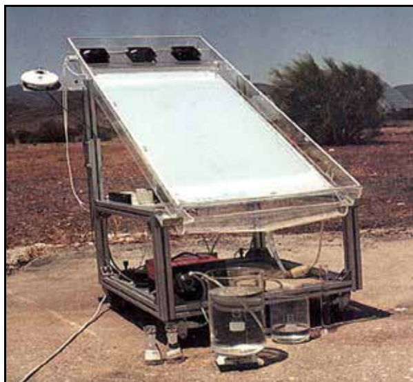
Fig. 2. A TFFBR installed at the PSA in Spain (Bockelmann et al., 1995)
