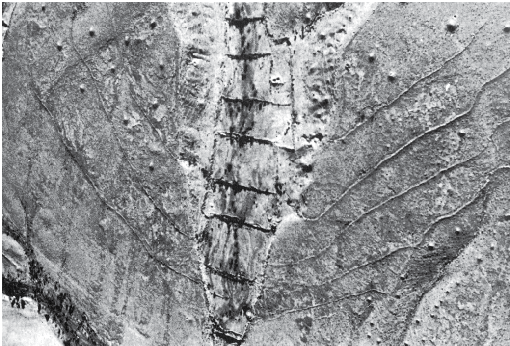
Fig. 1. Aerial photograph of a farm unit near Shivta in the Negev Desert. A terraced wadi and stone conduits leading runoff from hillsides to terraces are visible (after Evenari et al., 1982)
