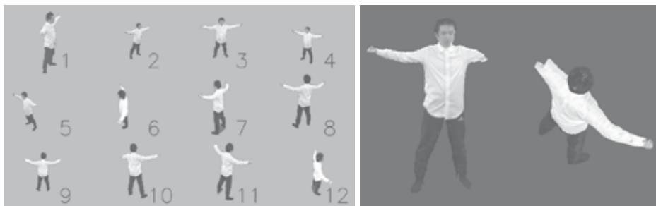
(a) Error in silhouette extraction only in camera #10. (b) Generated 3D model in which the left arm was not reconstructed properly.
