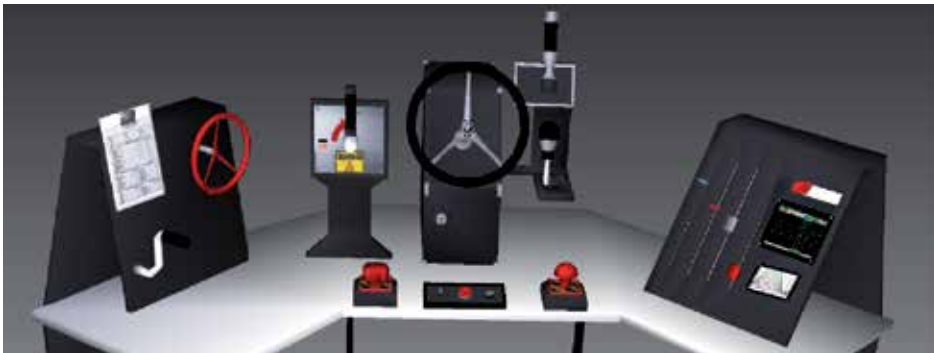
Fig. 1. Selection of control actuators defined in the European standard EN 894-3.
