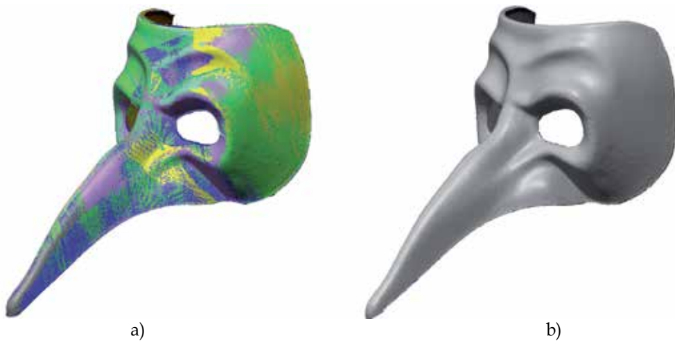
Fig. 10. Mesh generation: a) set of ICP aligned range maps. Different colours indicate the individual range maps; b) merge of all range maps in a single polygonal mesh.
