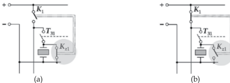
Fig. 20. The method of crosstalk elimination in a column of the active matrix using additional switches K_{zy} : (a) short-circuiting an inactive transducer, (b) open-circuiting when activating a transducer
