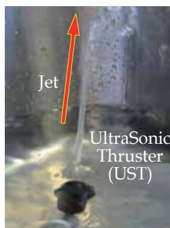
Fig. 1. An ultrasonic thrusters (UST) directing a jet through the free water surface.
