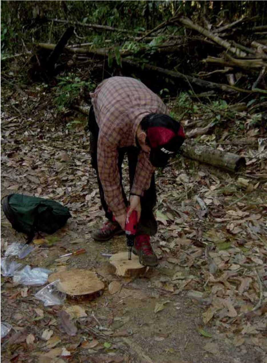
Image 2. Density measurements using a plug and tenon extractor attached to a hand-held power drill. Section of necromass sampled along a line intercept with section of fallen necromass being chain sawn into section for extraction.
