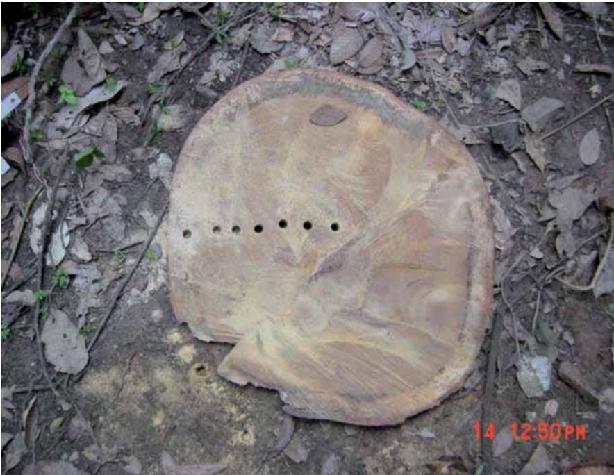
Image 3. Multiple samples extracted from a section of fallen necromass using the tenon extractor.
