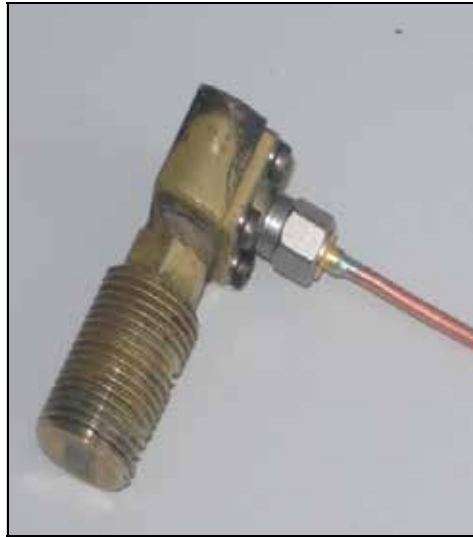
Fig. 20. The antenna for the PIT microwave sensor
