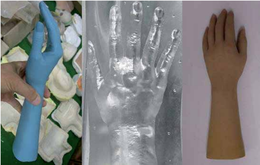
Fig. 10. The mock-up, mold and finished artificial hand skin
