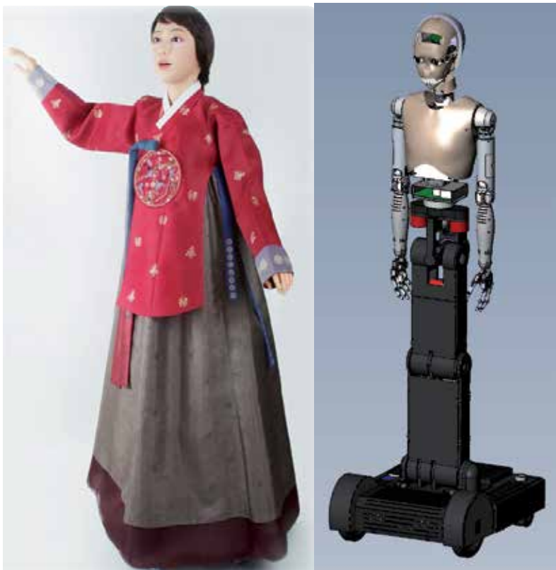
Fig. 1. The android robot EveR 3 and its mechanical drawing.
