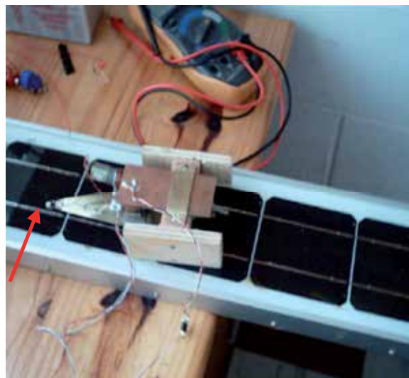
Fig. 3. Flux distribution profile apparatus resting on module string.
