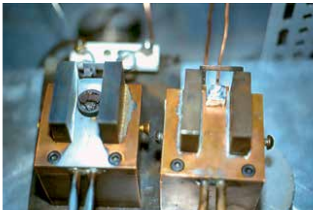
Fig. 2. Close-up photography of the two electron guns
