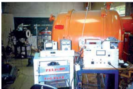
Fig. 1. Photograph of vacuum chamber, high voltage source, and vacuum gauges
