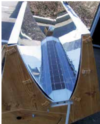
Fig. 1. Truncated CPC with 10 cell module string
