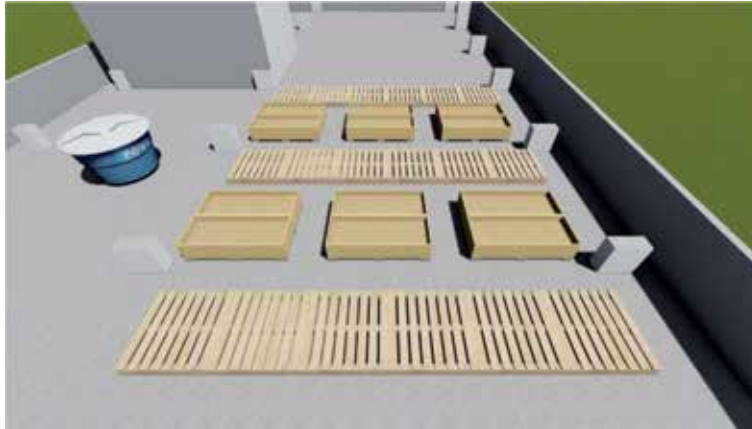
Figure 4. Gardens on roofs utilizing pallets.
