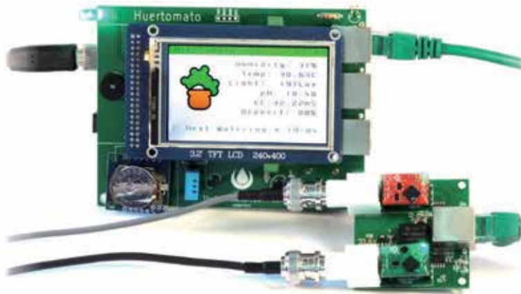
Figure 3. Huertomato microcontroller for measuring of humidity, water and air temperature, light, pH, electrical conductivity (courtesy of Arduino).
