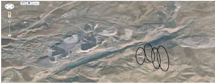
Figure 10. Free rock slide and falling site in Şırnak Asphaltite open quarry No 2, satellite view 1/18000.
