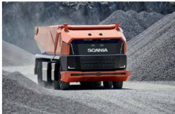
Figure 7. Autonomous driving Scania truck working in a closed area.
