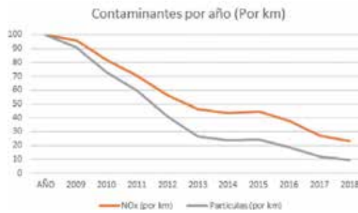
Figure 15. Evolution of NO x and PM emissions according to the EMT fleet.
