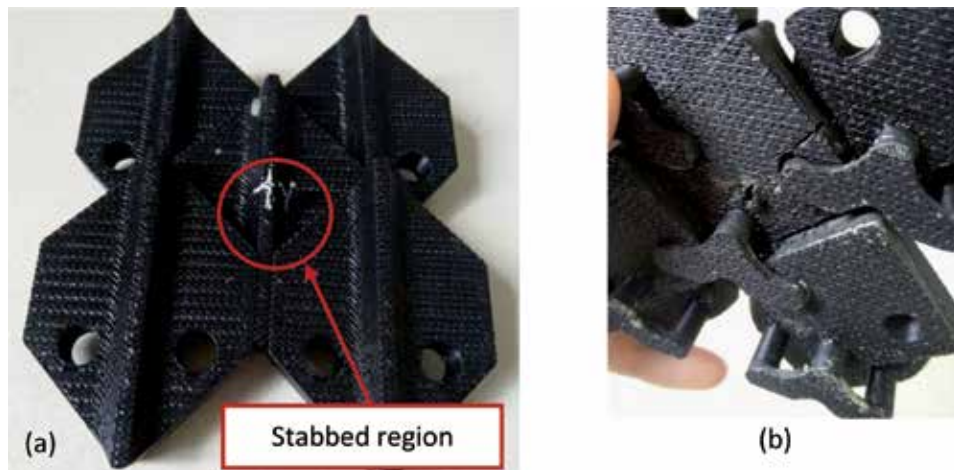
Figure 11. Stab test result of D4 specimen from (a) top and (b) bottom view.
