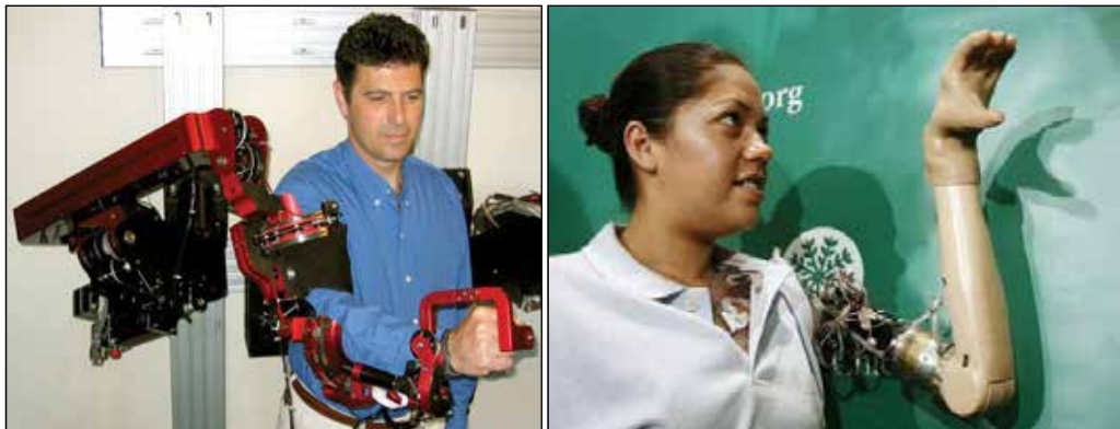
Fig. 1. (Left), orthotic robot of upper parts (Perry et al., 2007). (Right), prosthetic robot of upper parts (Rehabilitation Institute of Chicago, 2006)
