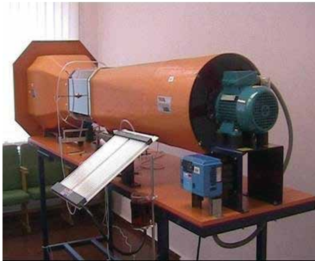
Fig. 17. Subsonic wind tunnel used for experiments at Mechanics Institute of Riga TU
