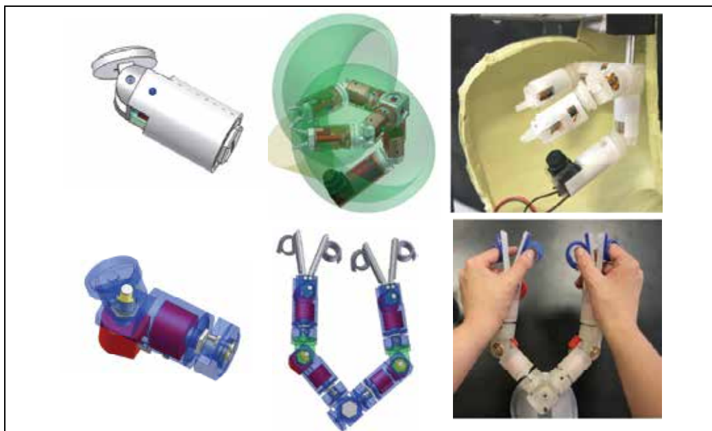
Fig. 6. Robotic modules (top line) and the reconfigurable master device (bottom line): one module (left), assembled modules (middle) and prototypes (right)
