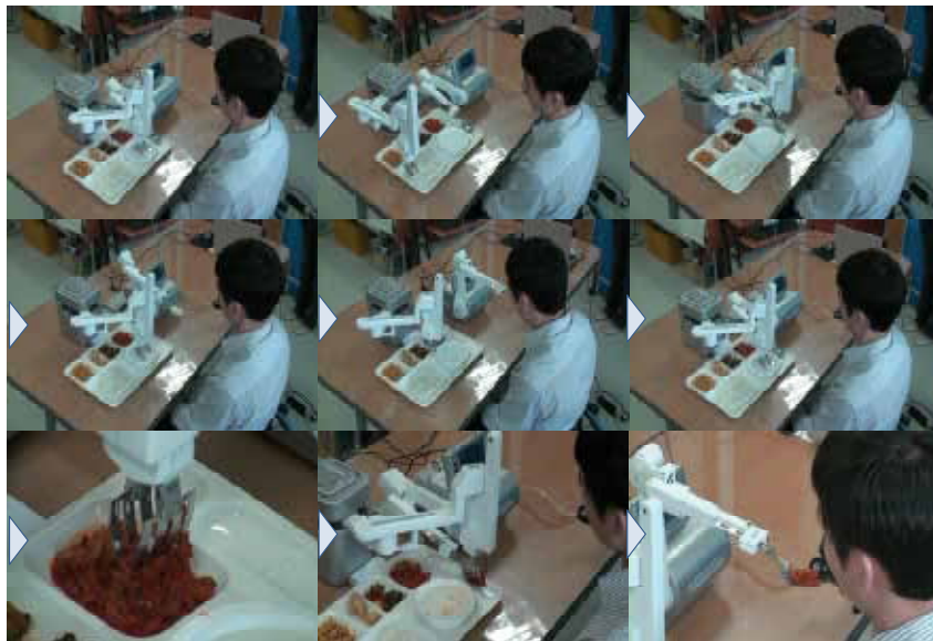
Fig. 12. The sequential motions of the self-feeding robot in dual-arm configuration. From the top left-hand side, the robot puts a gripper into a bowl of water and then grasps rice
