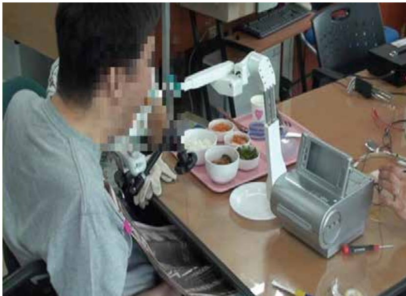
Fig. 14. The motions of the self-feeding robot in single-arm configuration. The caregiver picks food up on the spoon of the self-feeding robot, and then the user presses the button to receive the food
