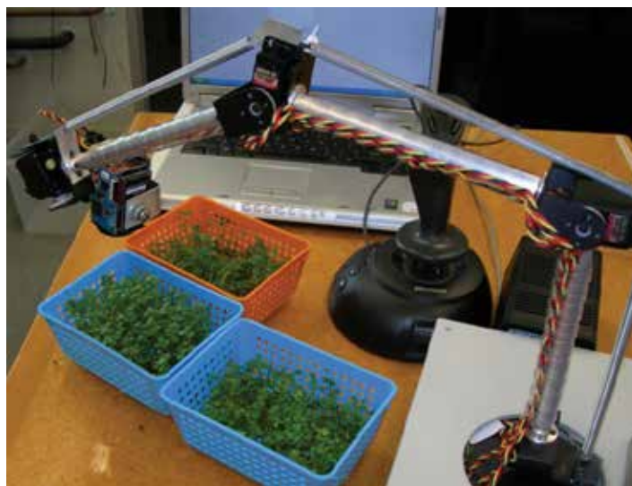
Fig. 3. The completed robotic arm with camera, joystick and plant trays
