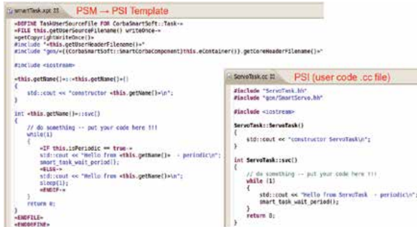
Fig. 17. PSM to PSI transformation of the SMARTTASK. Left : Excerpt of the transformation template ( xPand ) generating the PSI of a standard task. Right : The generated code where the user adds the business logic of the task.
