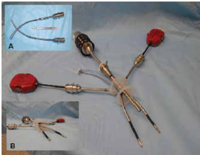
Fig. 5. VeSPA instruments and accessories. (A) Curved cannulae; (B) multichannel single-port, 8.5-mm robotic scope, flexible instruments passed through the cannulae
