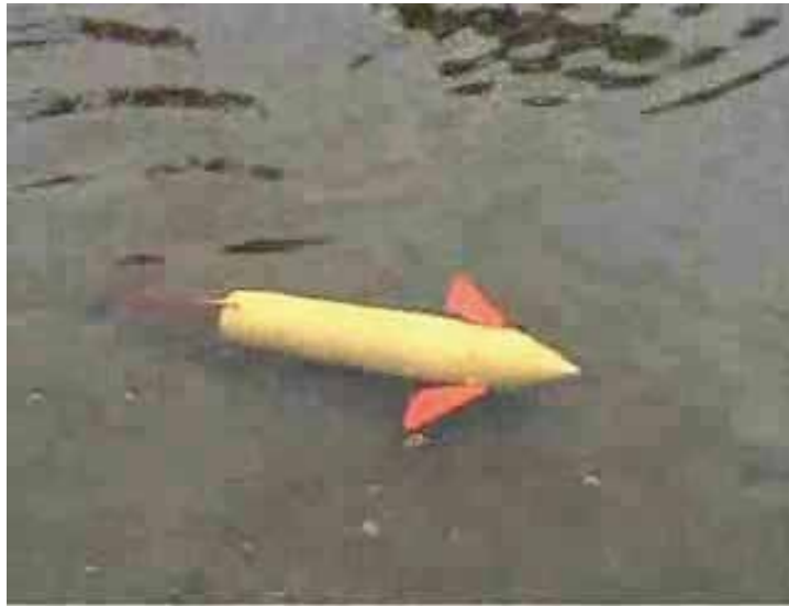
Fig. 34. Prototype was investigated in a large storage lake with autonomy power pack and distance control system, moving in real under water conditions with waves
