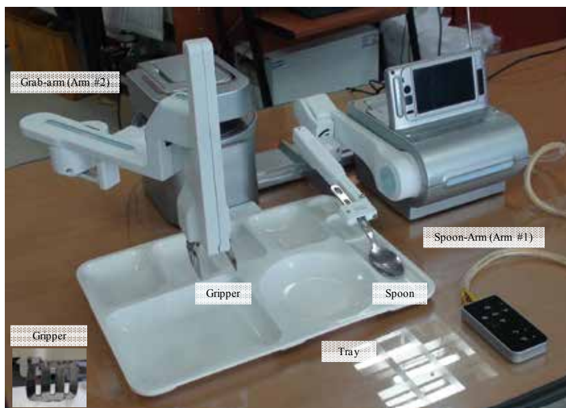
Fig. 4. Assistive robot for self-feeding. Spoon-arm (Arm #1) uses a spoon to transfer the food from a container to a user's mouth. Grab-arm (Arm #2) picks up the food from a container and then loads it onto the spoon of Arm #1
