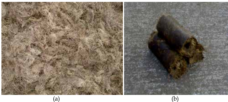
Fig. 9. PEFB before (a) and after (b) pelletizing
