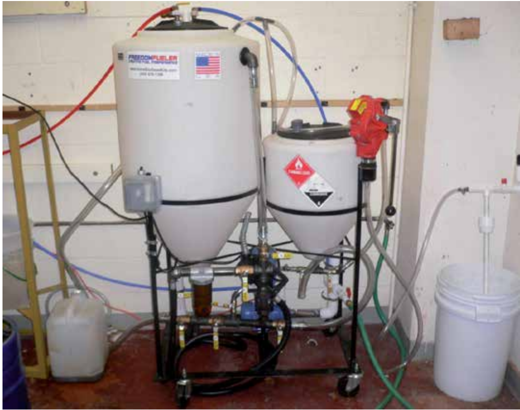
Fig. 3. Biodiesel Processor with a capacity of 40 gallons/day
