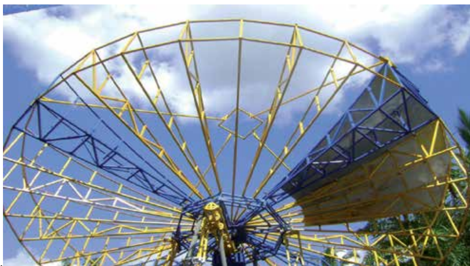
Fig. 8. A Parabolic Concentrator Heliostat (Source DIT-R&PGS-2011)
