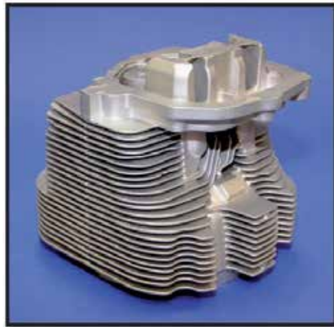
Figure 10. Air cooled cylinder head poured from Al-Ce binary alloy.
