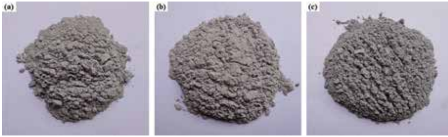
Figure 8. The cement clinker of autogenously pulverizable slag. (a) R = 3.60 , (b) R = 3.85 , (c) R = 4.10 .
