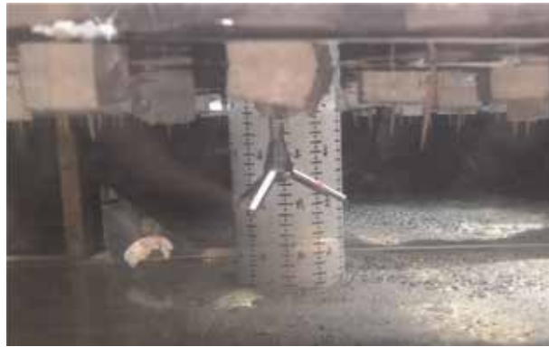
Figure 9. The ADV measurement around the bridge piers under rough ice-covered condition.
