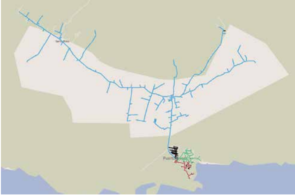
Figure 3. Medium voltage distribution system in Santa Cruz [30].
