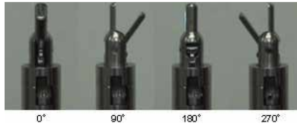
Fig. 9. Transition chart of the rotary gripper
