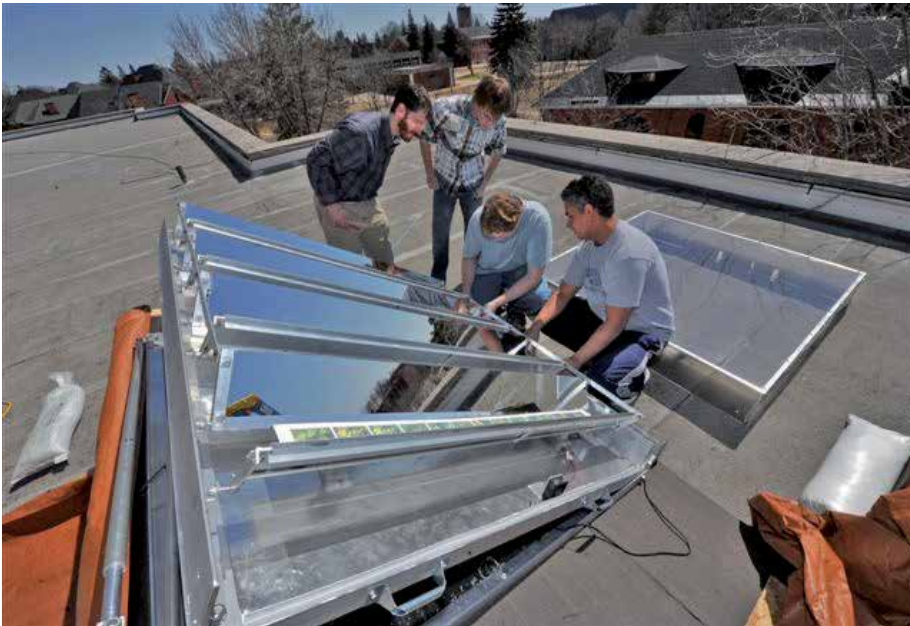
Fig. 10. Single-axis solar louver tracking design with 3M brand Cool Mirror (photo courtesy of Lake Superior State University).
