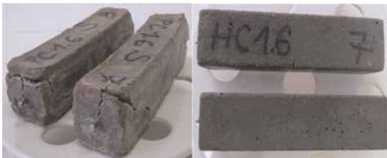
Figure 15. Destroyed integrity of PC mortar after 4 years of aggressive attack with sodium sulphate (left) and intact state of H-cement after 5 years of aggressive attack of 5% wt. Na 2 SO 4 (right).
