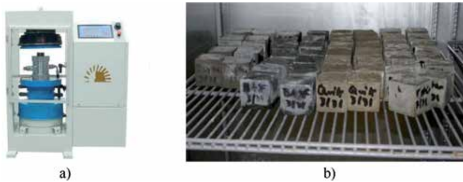
Figure 3. (a) Compressive test machinery. (b) Cube concrete samples.
