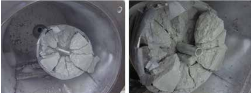
Figure 12. 8000 psi cylinder impacted by 30 mm diameter and 218 g projectile at v = 360 m/s.
