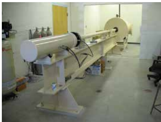
Figure 5. Gas operated facility for testing concrete samples.
