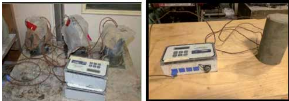
Figure 5. The maturity-meter device used for concrete strength evaluation.
