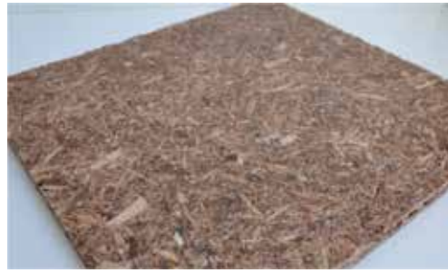
Figure 8. Tannin resin adhesives for manufacturing particleboard.
