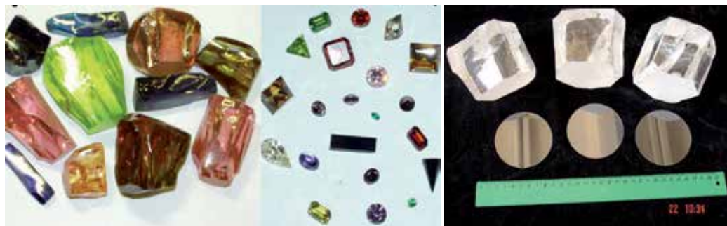
Fig. 1. Great color variety of the crystals combined with unique optical properties makes fianite single crystals a promising material for jewellery, arts and Crafts (left); fianite substrates 3" in diameter (right).
