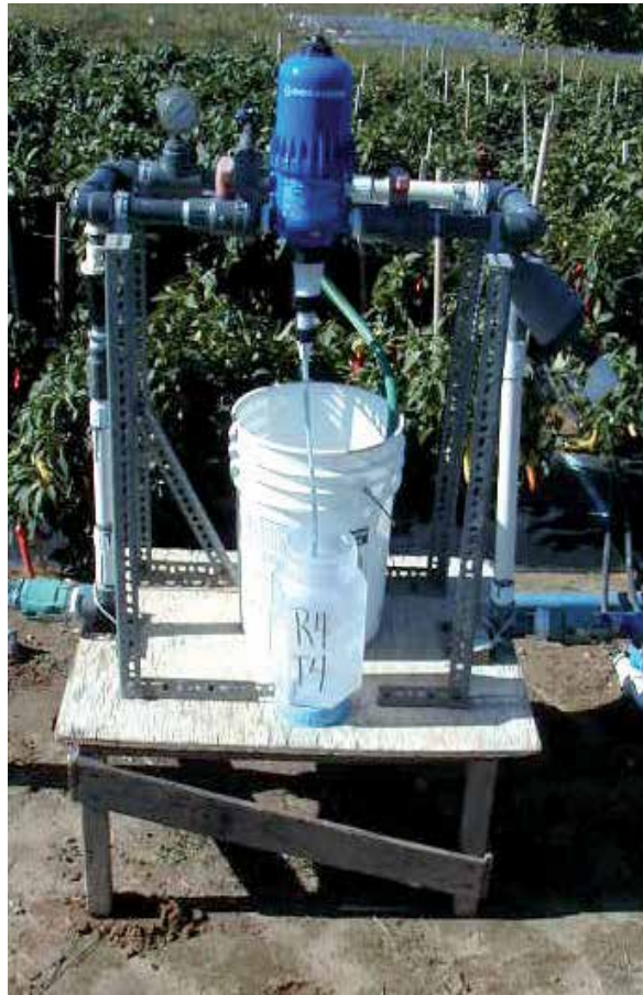
Fig. 5. A Dosatron ® injection pump injecting a pesticide in bell pepper, Bridgeton, NJ.
