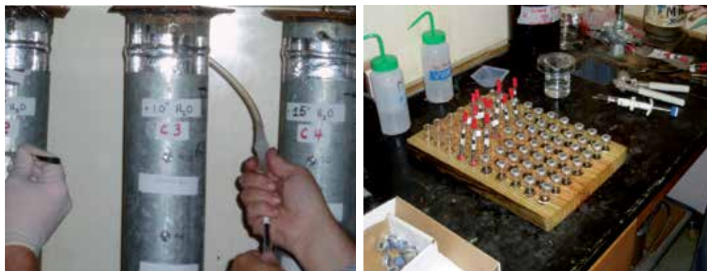
Fig. 2a. Charcoal filters replaced periodically. Fig. 2b. Charcoal filter extracted into vials.
