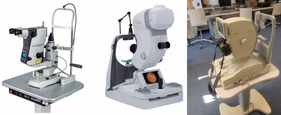
Figure 3. Slit lamp example (left) [6]; example of a non-mydratric fundus camera (middle) [7]; (right) fundus camera used in the biometric laboratory at FIT BUT (right).
