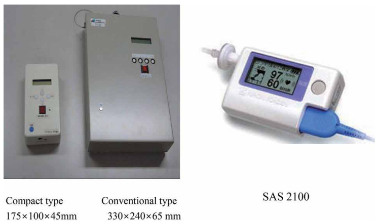
Figure 20. Comparison of compact F-SAS sensor and conventional one (left) and SAS 2100 (right).
