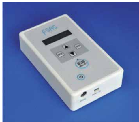
Figure 16. Compact F-SAS sensor system (175 × 100 × 45 mm, 390 g, voltaic drive during electric outage) (after improvement).
