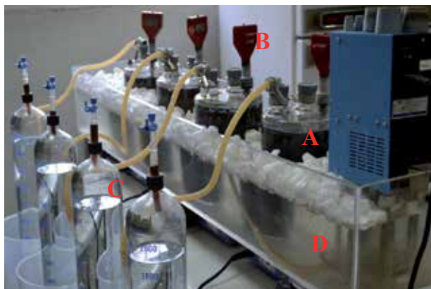
Fig. 1. Experimental laboratory scale anaerobic reactors (A: reactor, B: pH-meter, C: gasometer with NaOH for methane measurement, D: water bath for temperature control).
