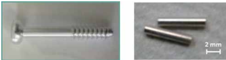
Figure 2. Screws (left image) and cylindrical pins (right image) are often used in orthopedic and trauma research.
