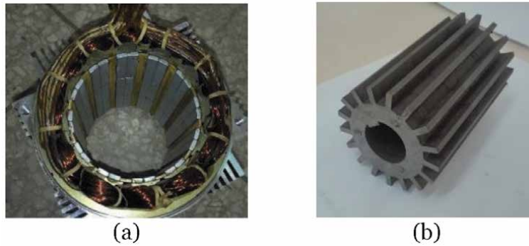
Figure 28. 12-slot/17-pole FRPMM prototype: (a) stator; (b) rotor.
