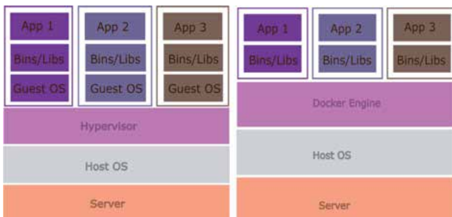
Figure 1. An illustration showing the architectures of virtualization technologies: hypervisor-based virtualization (left) and container-based virtualization (right) [2].
