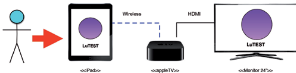
Figure 2. Architecture for LuTEST. This application makes a DUI using a Tablet iPad and an Apple TV.
