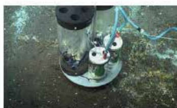
The IronMan chemical analyser deployed on small cracks.
