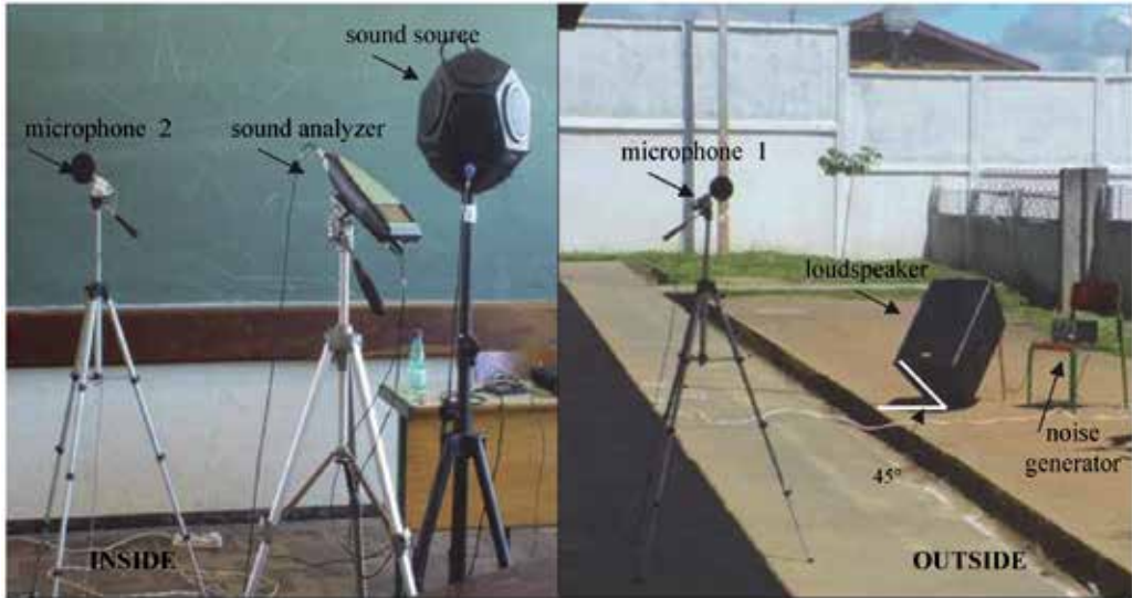
Fig. 2. Measurement of façade insulation according to ISO 140-5 10
