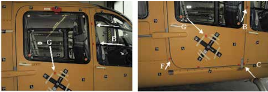
Fig. 17. Leakage points (in red) on the helicopter cabin found by means of the ultrasound technique (cabin right panels)
