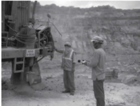
Fig. 15. Sound measurement during drilling
