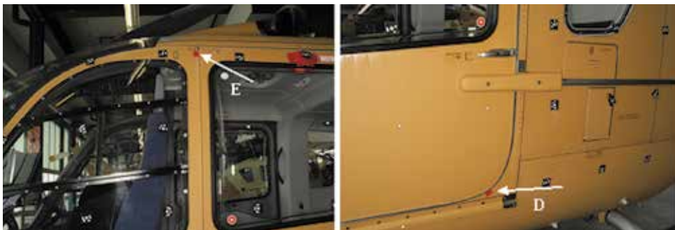
Fig. 18. Leakage points (in red) on the helicopter cabin found by means of the ultrasound technique (cabin left panels).
