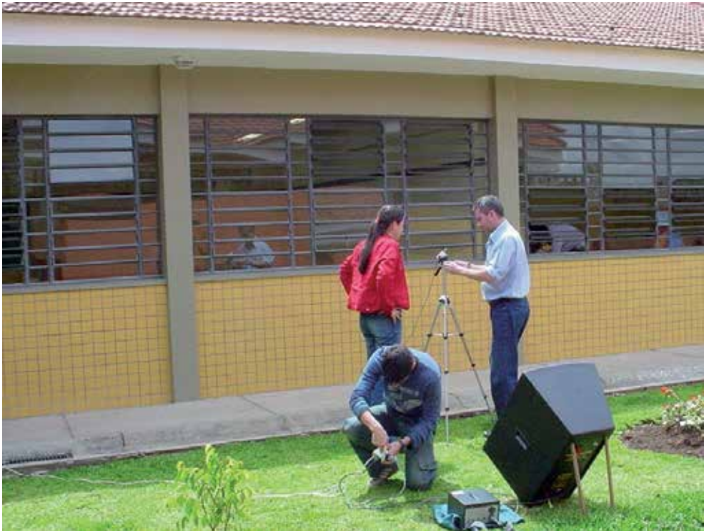
Fig. 16. Measurement of the sound insulation of the façade according to ISO 140-5 10 (Luarlindo dos Reis Borges School)
