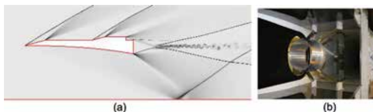
Figure 7. (a) Freestanding conical shock at center line, produced by axisymmetric Busemann leading edge annulus in a Mach 3 freestream. CFD calculation by E.V. Timofeev. (b) Busemann leading edge annulus in Mach 3 wind tunnel at DRDC [40].
