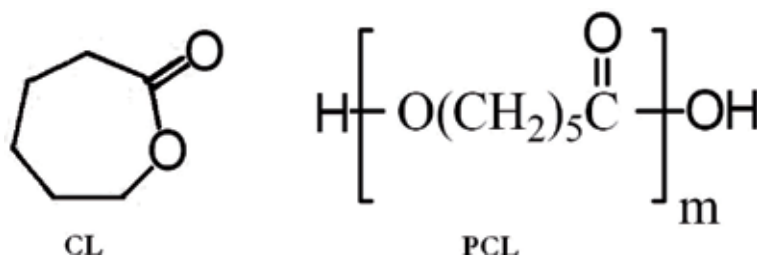
Figure 5. Molecular scheme of ε-caprolactone as oligomer and poly(ε-caprolactone) as homopolymer.
