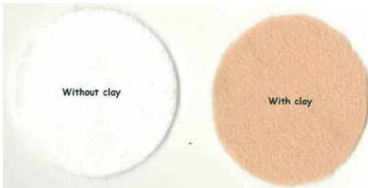
Figure 15. Clay added geotextile to improve adsorption efficiency.
