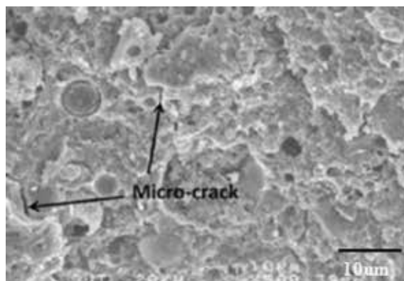
Figure 7. SEM micrograph clay-based geopolymer brick cured at 85 Celsius for 24 hours [11].
