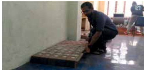
Figure 3. Dimensionality test of geopolymer bricks.
