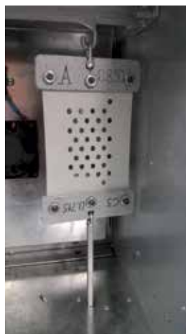
Figure 2. Placement of the sample to the upper and lower jaws.
