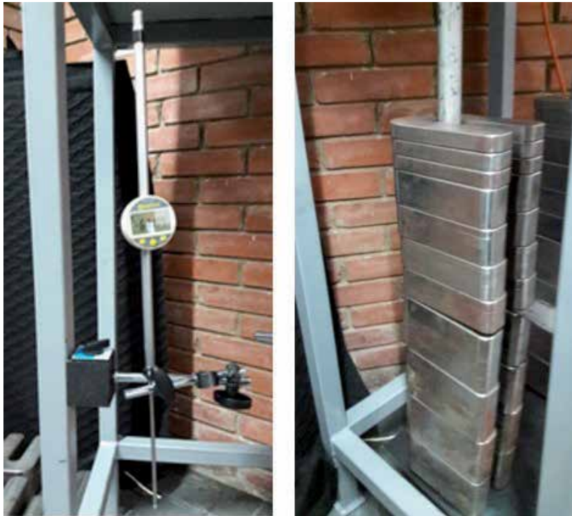
Figure 4. Deformimeters in the base of the oven (left) and placement of weights in the stems (right).
