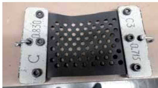
Figure 2. Placement of the sample to the upper and lower jaws.
