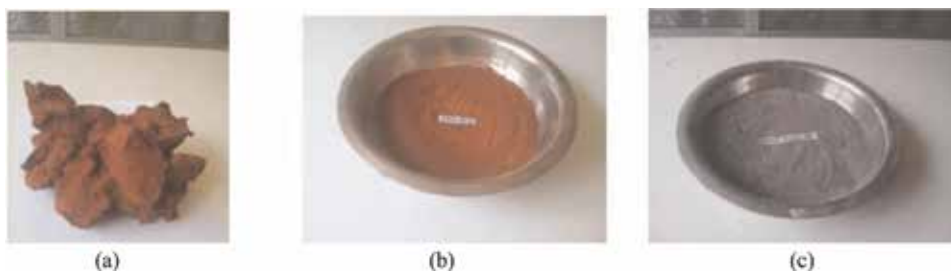
Figure 4. (a) RM oven dried (b) RM ground (c) rice husk ash.
