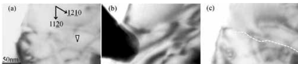
Fig. 8. A preliminary result for in-situ examination of a photo-induced glide of an individual dislocation in ZnO. TEM images of the screw dislocation indicated with the arrowhead in (a); before (a), under (b), and after (c) the illumination of a near-field light with photon energy of 2.41 eV. The broken curve in (c) indicates the dislocation line before the illumination. (Ohno, 2010a)
