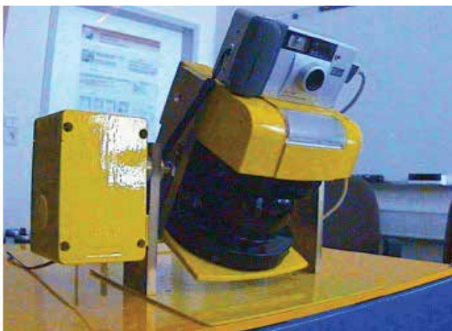
Fig. 15. A 3D laser range finder for autonomous mobile robots. The servo is mounted at the left side. A camera on top is used to get texture images for the realistic appearances of a 3D scene (Surmann at al. 2001)
