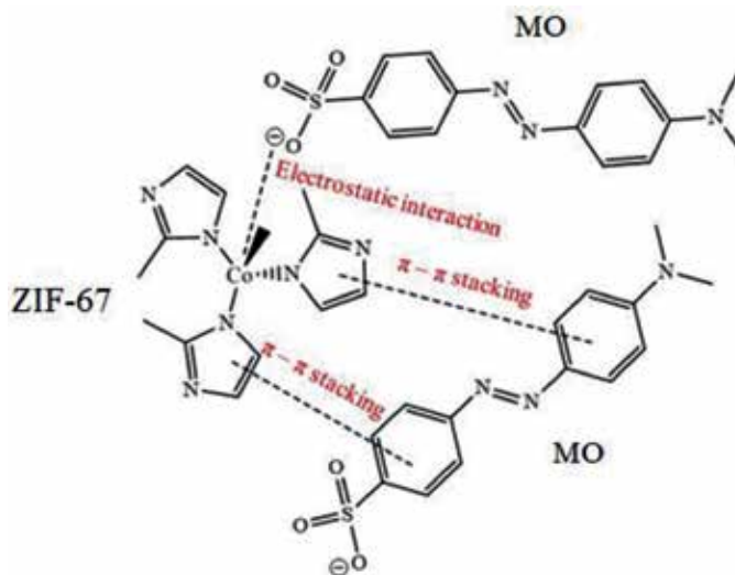
Figure 10. Mechanism of MO adsorption to ZIF-67.
