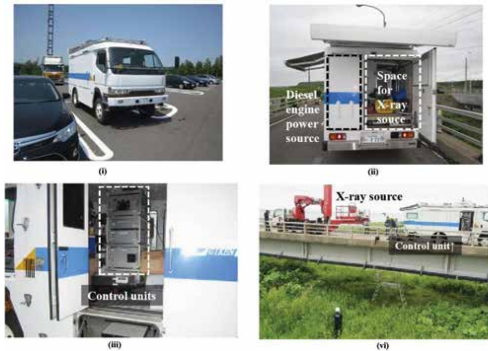
Figure 17. Special inspection car for the 950 keV/3.95 MeV X-ray sources. (i) Front view, (ii) Back view, (iii) Control units, and (iv) On site set-up.
