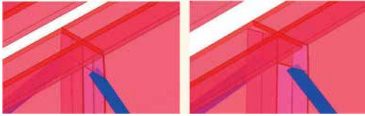
Figure 12. Skewed (right) and non-skewed (left) connection plates.
