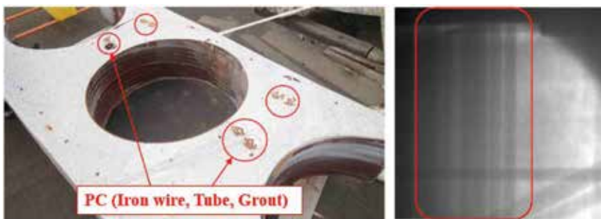
Figure 8. Cut sample from a hollow flow bar-type bridge and X-ray transmission image acquired by the 3.95 MeV X-ray source. The total thickness of the concrete where the X-rays penetrate is ~400 mm. Several PC wires located deep in concrete are visualized.
