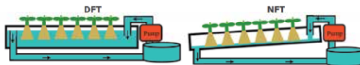
Fig. 9. Hydroponic production with deep flow technique (DFT) and nutrient film technique (NFT).
