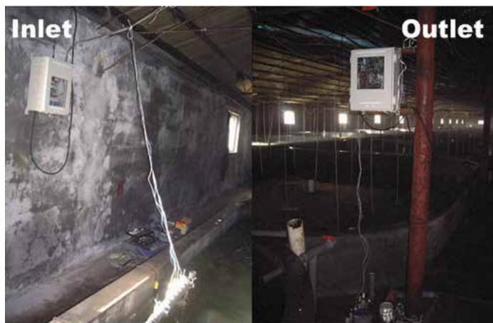
Fig. 7. Water quality dynamic monitoring systems installed in an aquaculture farm.
