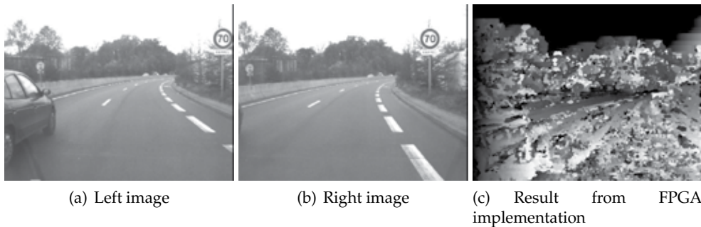
Fig. 4. Stereo images acquired from a vehicle in the highway: a) left image b) right image and c) the disparity map.
