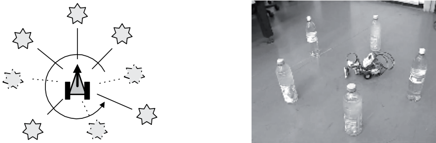
Fig. 3. The mobile robot with ultra-sonic sensor acting in the stochastic environment: after collision, the obstacle randomly changes its location in the environment.
