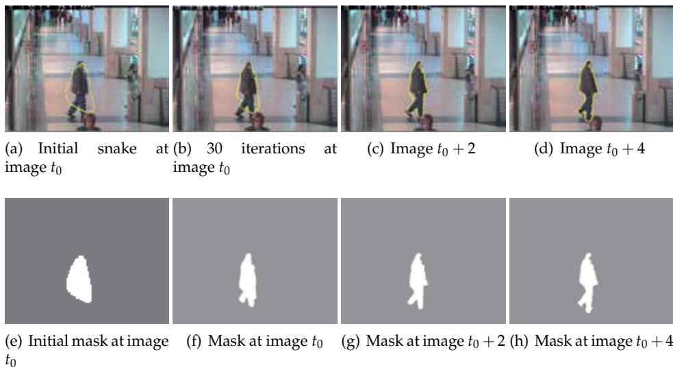
Fig. 10. Results of the detection and tracking of a non-rigid dynamic object, in this case a pedestrian on the same sequence of figure 9. Here, we have processed 5 consecutive images, executing 30 iterations per image in order to find the actual object shape.
