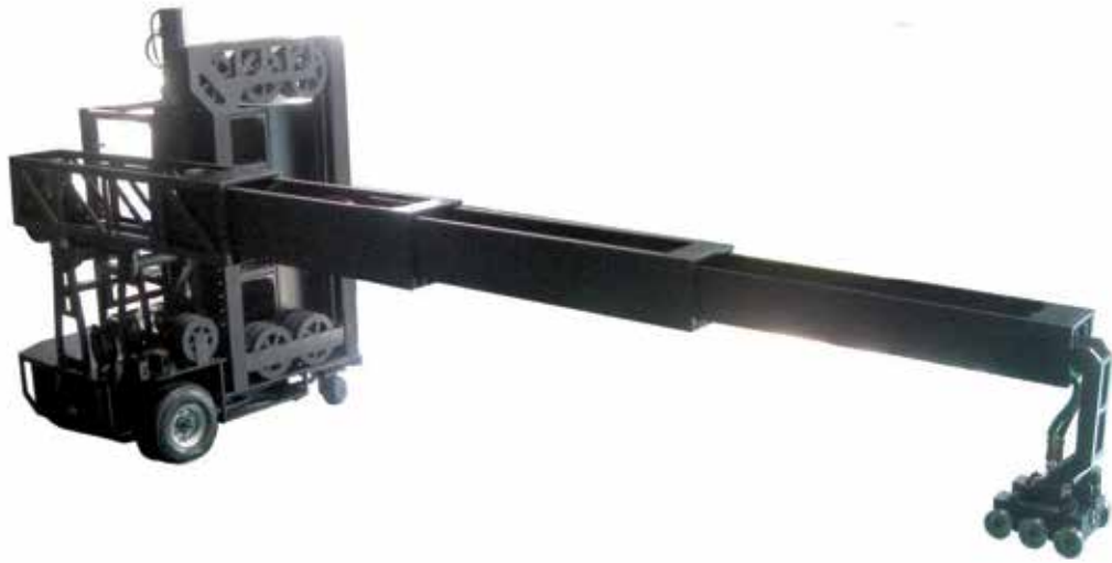
Fig. 2. APSCR stretches its arm up to 3.8 m.
