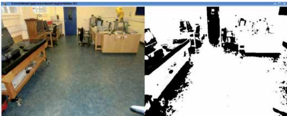
Fig. 3. Appearance based obstacle detection method.
