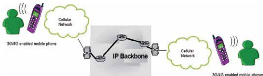
Fig. 4. 3G/4G wireless VoIP call path
