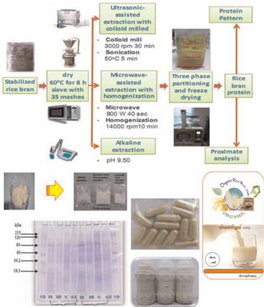
Figure 17. Different methods for extraction of protein from rice bran. Sources: Phongthai et al. [62], Phongthai et al. [63], and Phongthai et al. [64].
