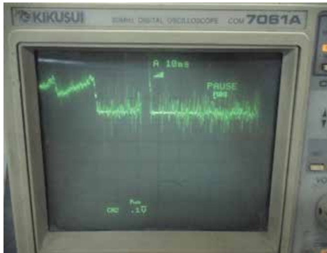
Fig. 7 a. Snap shot of online time varying ECSMM process current during glass pellet micromachining.
