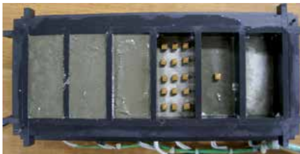
(b) zig structure for the concrete blocks fabrication
