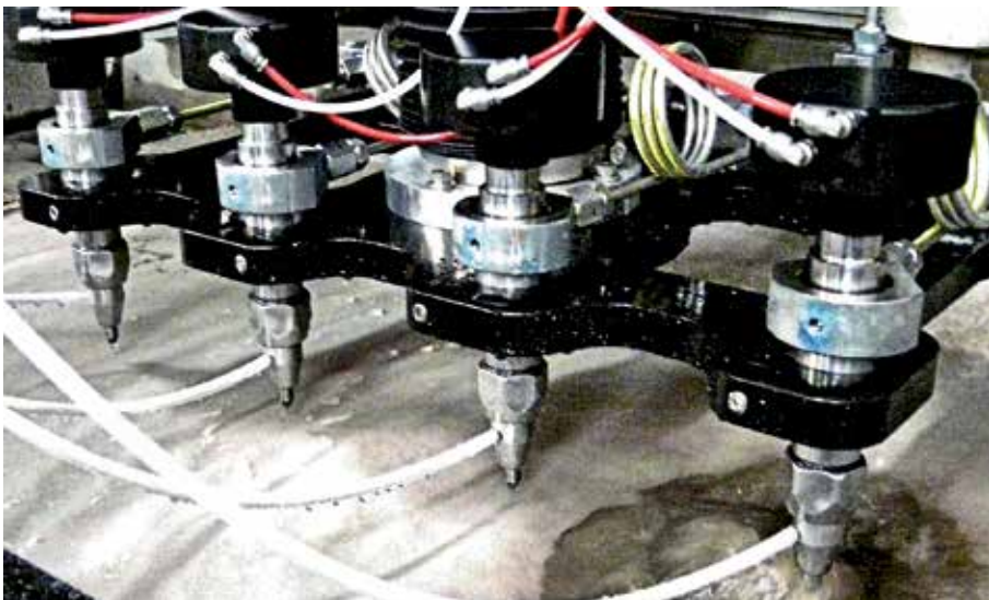
Fig. 25. Four nozzles mounted on a platform for increased productivity (Liu et al., 2011b)
