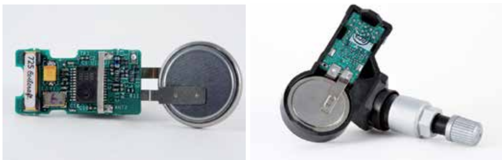
Fig. 24. Complete system fitted with the valve and a wireless communication system (reproduced with kind permission Janusz Bryzek).
