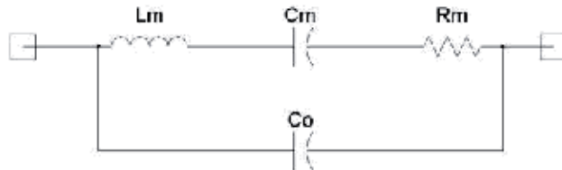
Fig. 10. FBAR equivalent circuit, where L_m is the motional mass, C_m is the motional capacitance, R_m is the motional resistance and C_0 is the static capacitance.
