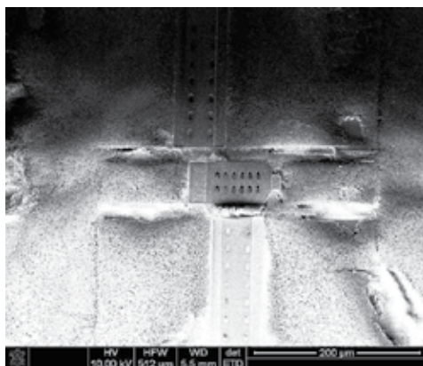
Fig. 10. SEM of the RF MEMS switch with supporting layer
