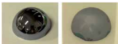
Fig. 4. Photos of the hemisphere specimen: (a) before etching and (b) after etching (etching temperature = 61 °C).
