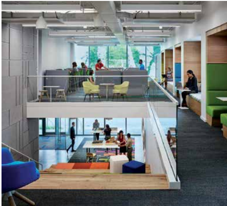
Figure 3. Interface Headquarters in Atlanta, Georgia, USA. A combination of acoustic solutions used: separate acoustic zoning, quieter background noise from chilled beam system, mechanical sound tuned to sound masking pitch, and interior finishes and furnishings with acoustic properties. LEED platinum and WELL silver certifications pending. Photo courtesy: Nick Merrick, Hall + Merrick photographers.
